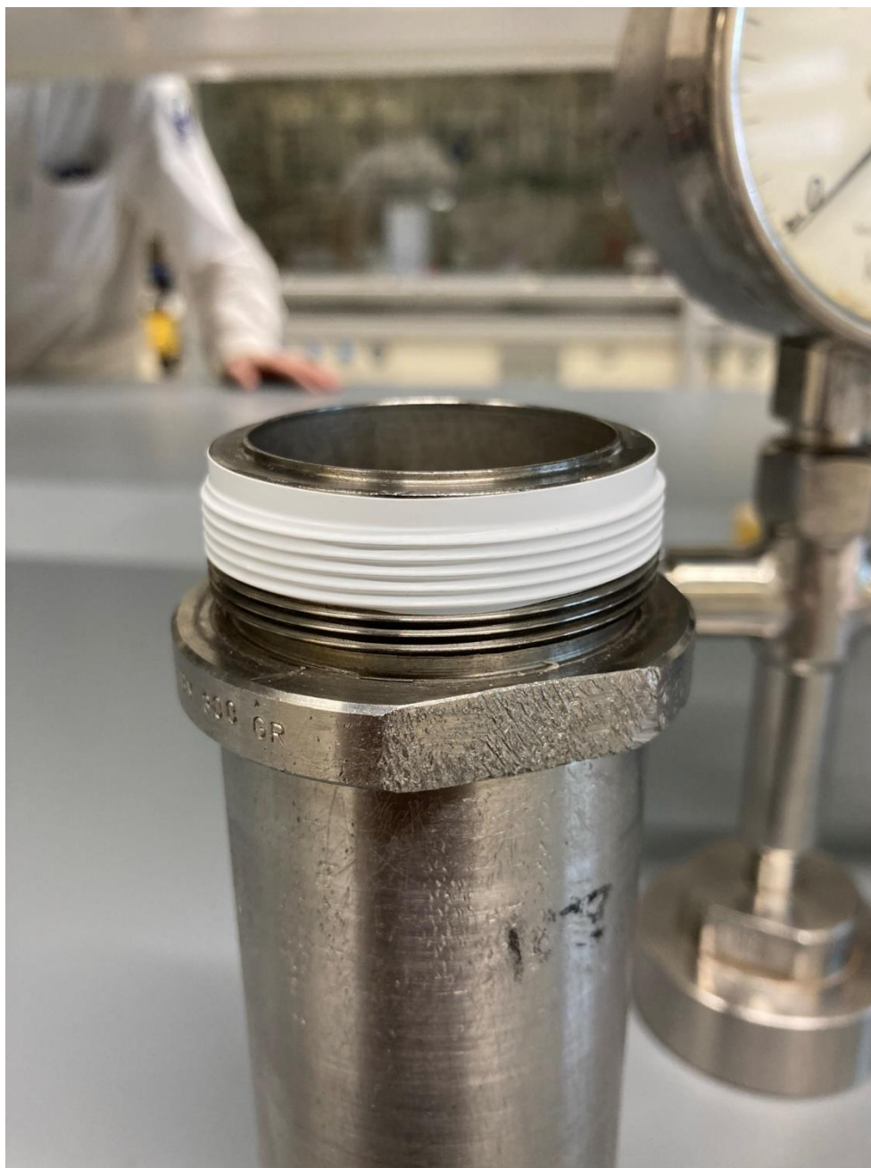
Figure 3: Teflon tape wrapped just to the edge of the opening
