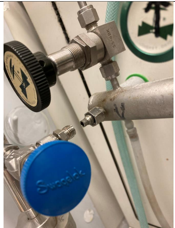
Figure 12: Connect the autoclave to the pressure outlet
