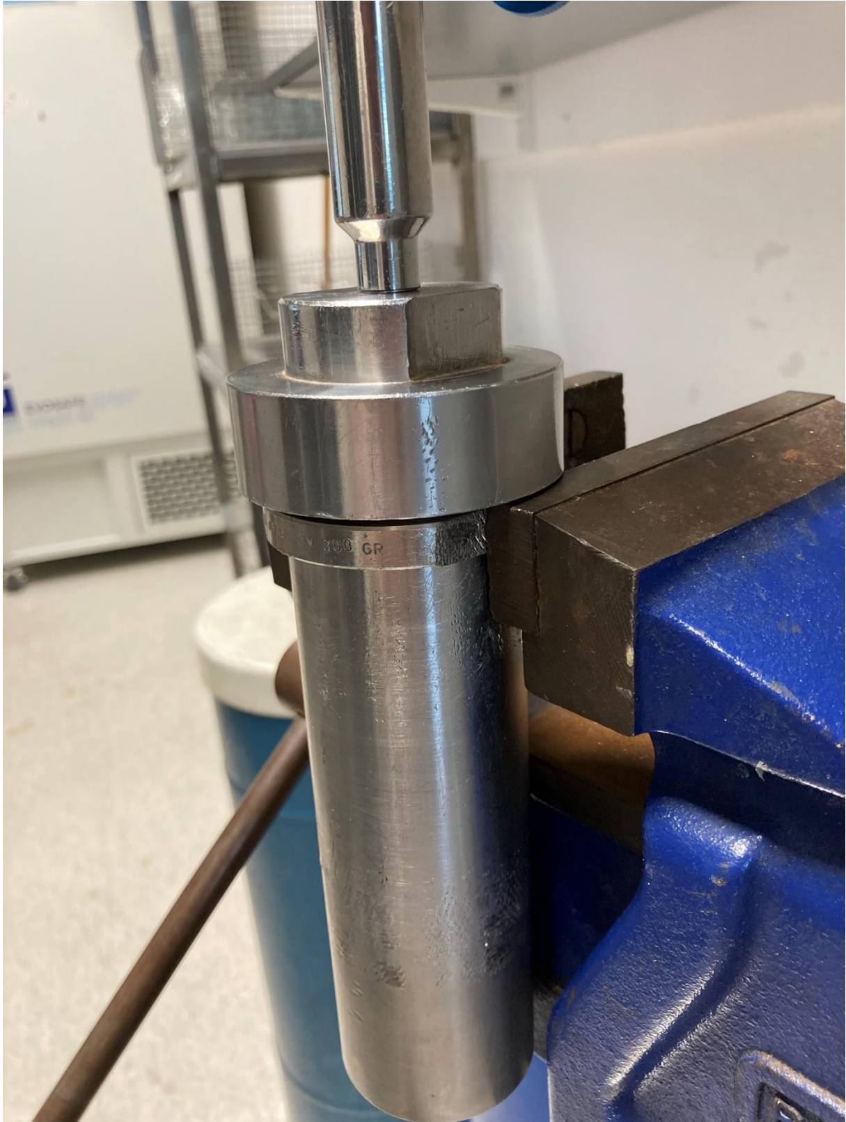
Figure 6: The autoclave is secured on the flat edges of the bottom part in the vice
